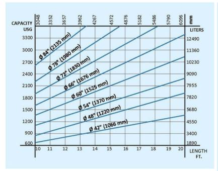
**Note:** When selecting dimension for storage vessel, determine first storage capacity and select the length of vessel to suit the available space. The resulting diameter is found at the intersection of capacity and lenght lines. For any other capacity not listed and/or other information please contact us. Maximum standard vessel available: 120" (3048 mm) dia. x 30' (9144 mm) long.
