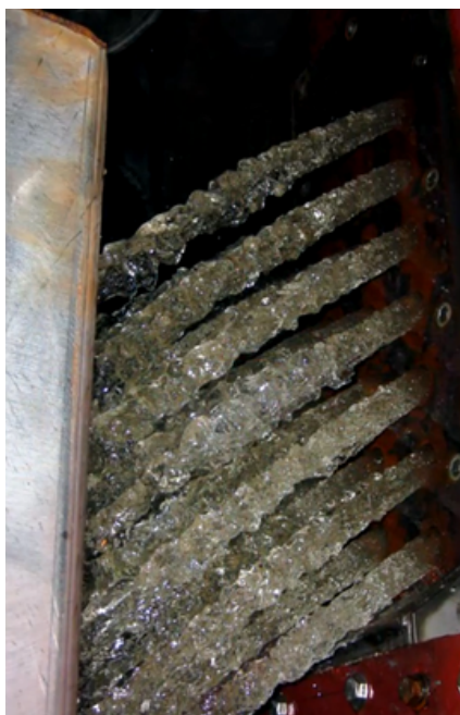
Parallel Water Jets - from Nozzle Stock to Electrode Target Plates
